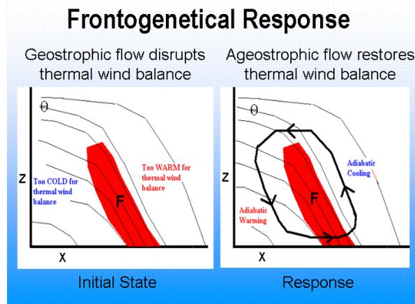
**Figure 7.** Cross-section showing the ageostrophic response to frontogenesis.
